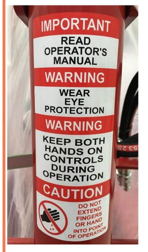
This safety decal is on the hydraulic ram and should be replaced if missing or becomes illegible.
