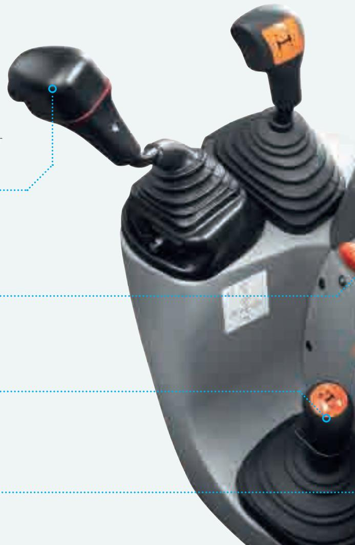
Intentional PTO switch, which must be selected to keep the PTO engaged when leaving the operators seat.
