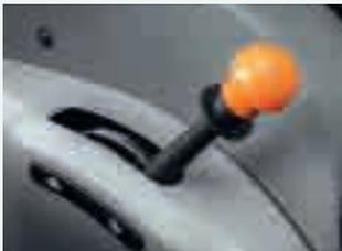
The ergonomically positioned creeper engagement lever falls naturally to hand (Creeper option only).
