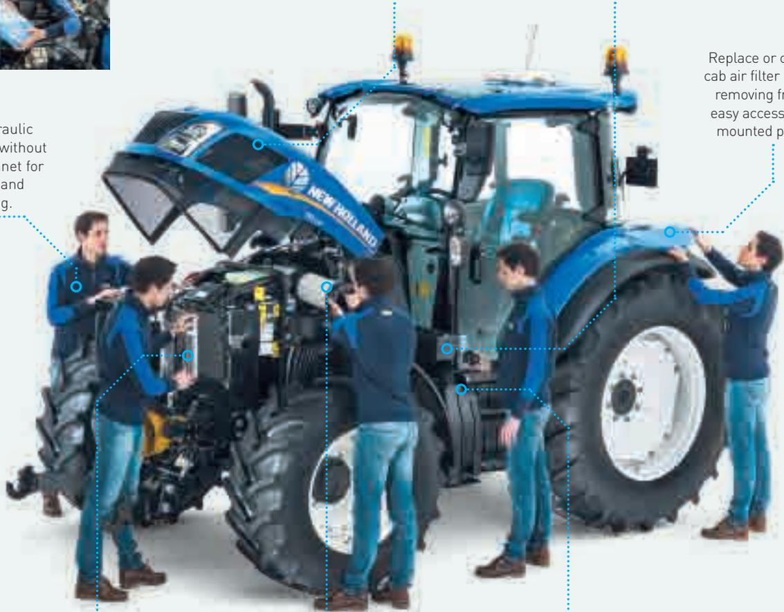
The cooling package slides out for simple and efficient cleaning.
